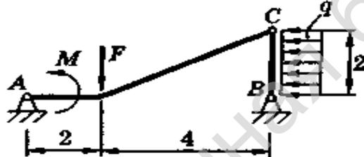
$M = 20 \text{ кН}\cdot\text{м}; q = 25 \text{ кН/м}; F = 40 \text{ кН}$
