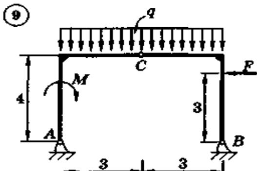
$M = 60 \text{ кН}\cdot\text{м}; q = 20 \text{ кН/м}; F = 30 \text{ кН}$
