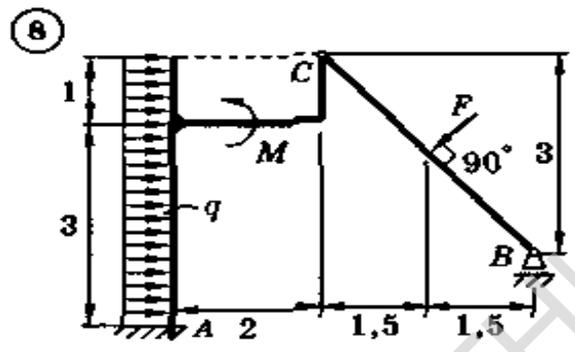
$M = 11 \text{ кН}\cdot\text{м}; q = 4 \text{ кН/м}; F = 13 \text{ кН}$
