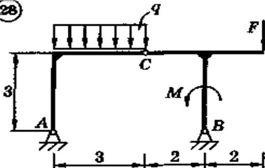
$M = 30 \text{ кН}\cdot\text{м}; q = 10 \text{ кН/м}; F = 50 \text{ кН}$
