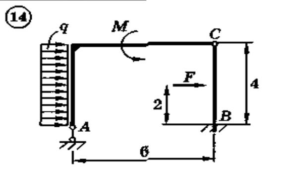
$M = 40 \text{ кН}\cdot\text{м}; q = 10 \text{ кН/м}; F = 30 \text{ кН}$
