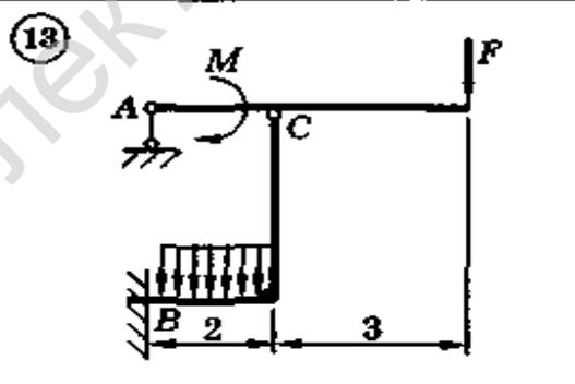
$M = 40 \text{ кН}\cdot\text{м}; q = 20 \text{ кН/м}; F = 20 \text{ кН}$
