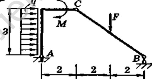
$M = 40 \text{ кН}\cdot\text{м}; q = 10 \text{ кН/м}; F = 30 \text{ кН}$
