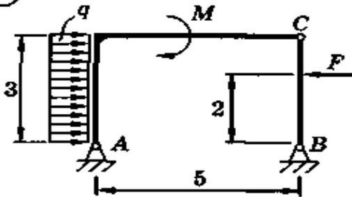
$M = 40 \text{ кН}\cdot\text{м}; q = 20 \text{ кН/м}; F = 60 \text{ кН}$
