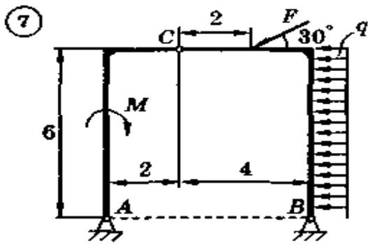
$M = 30 \text{ кН}\cdot\text{м}; q = 10 \text{ кН/м}; F = 15 \text{ кН}$
